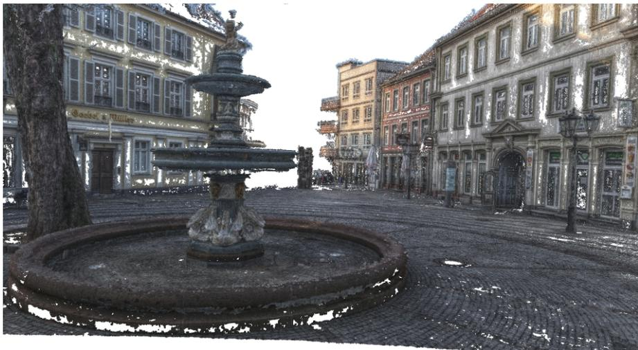
Figure 9. 3D reconstruction of a city place. Top: results of the structure from motion method. Middle and bottom: Dense point cloud generated using multiple view stereo with the calibrated cameras as input.
